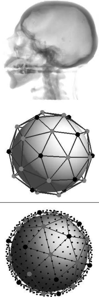
Figure 7: Vertices of regular icosahedron (black) and its dual dodecahedron (gray) are triangulated into 60 triangles (right, center), which are recursively subdivided (right, lower) to give points on the unit sphere that serve as quantized normal vectors.
